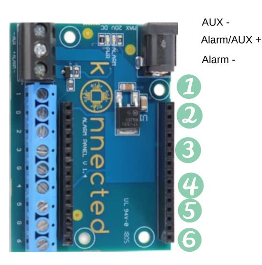
Ground is shared for 1-2 / 3-4 / 5-6-out Note: DO NOT exceed 3.3v for Konnected inputs Alarm panel can supply 1 amp
