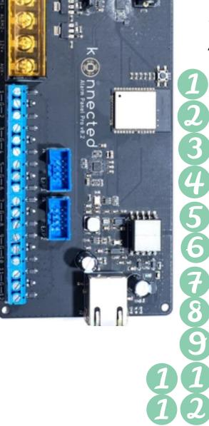
Ground is shared for 1-2 / 3-4 / 5-6-out Note: DO NOT exceed 3.3v for Konnected inputs PoE can supply 1 amp 12v
