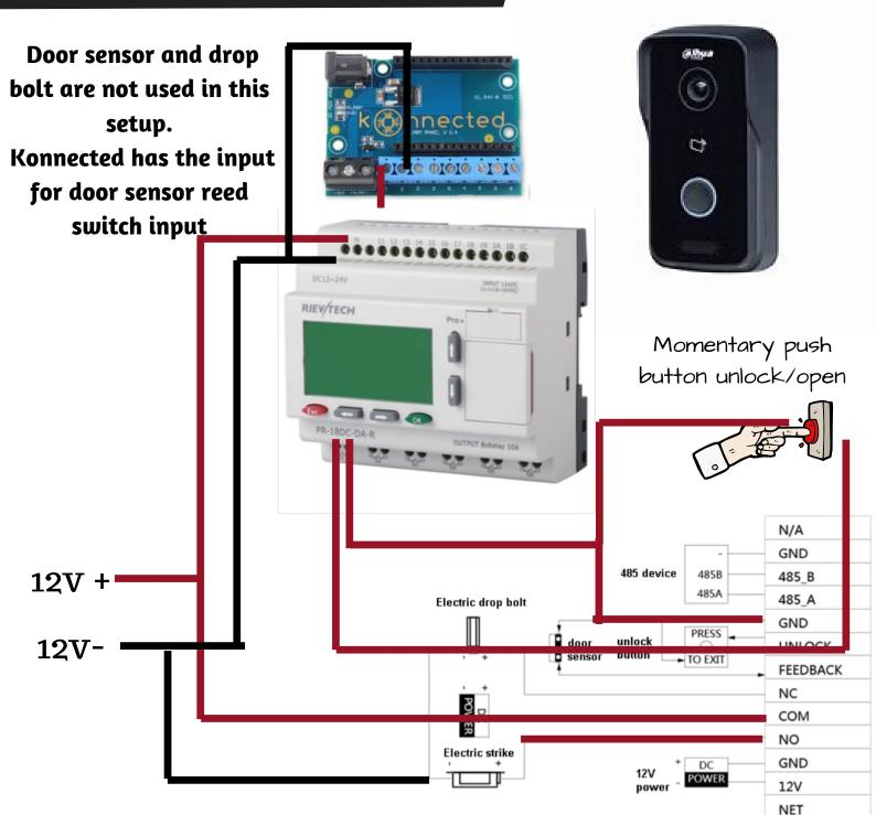
If PoE is used; 12v to VIP VTO is not needed. It is recommended to run 6 core security cable to front door to service mag-lock /door-sensor/open-button
